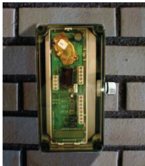
Figure 9: SenseAir's CO sensor mSENSE II in IP54 housing.
