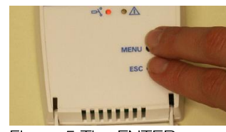
Figure 5 The ENTER command is done by pushing buttons MENU and ESC at the same time for about 14s.
