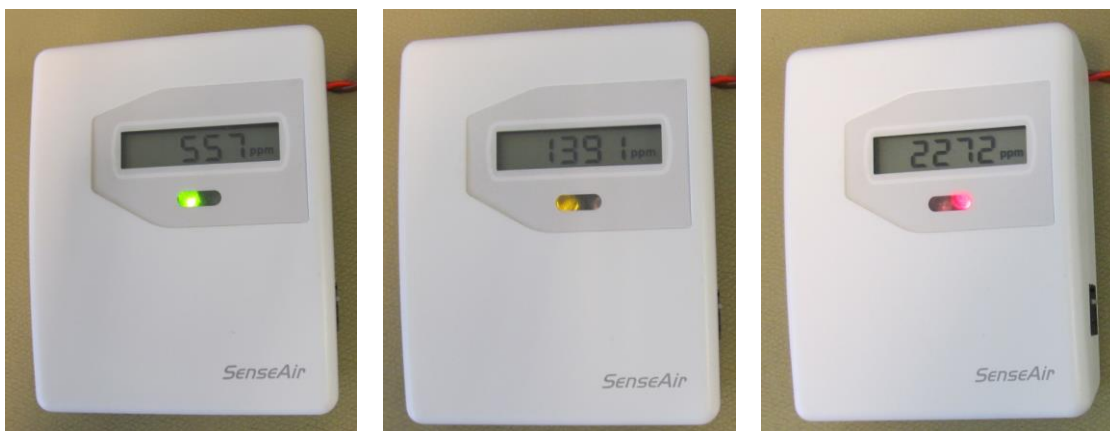
Figure 1 eSENSE FAI with the three LED indicating CO 2 levels
