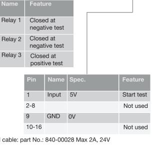
Signal cable: part No.: 840-00028 Max 2A, 24V
